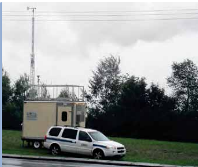
DELG's mobile air quality monitoring unit in Atholville, NB.
